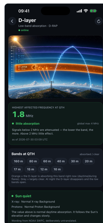
D-layer: highest affected frequency at the QTH, affected bands, solar situation.
