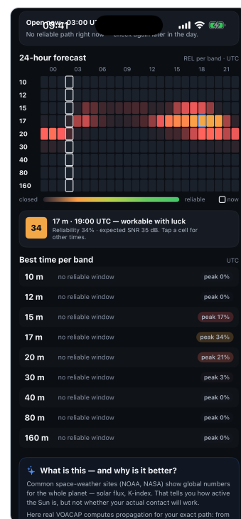
The 24-hour matrix. Green means dependable, red means very unlikely.
